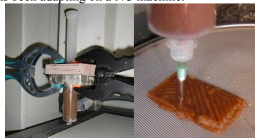
Fig 5. Second syringe experimentation with a wood pulp
